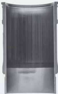
Severely Scuffed Liner
