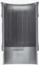
Severely Scuffed Liner
